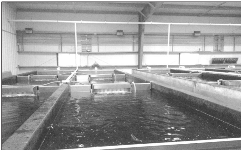
Medvejie installed an “Airlift” system to allow higher fish densities this summer in coho raceways. The system was integral in allowing us to rear both Medvejie and Sawmill Creek production while Sawmill was without water due to Sitka’s hydro expansion project.
