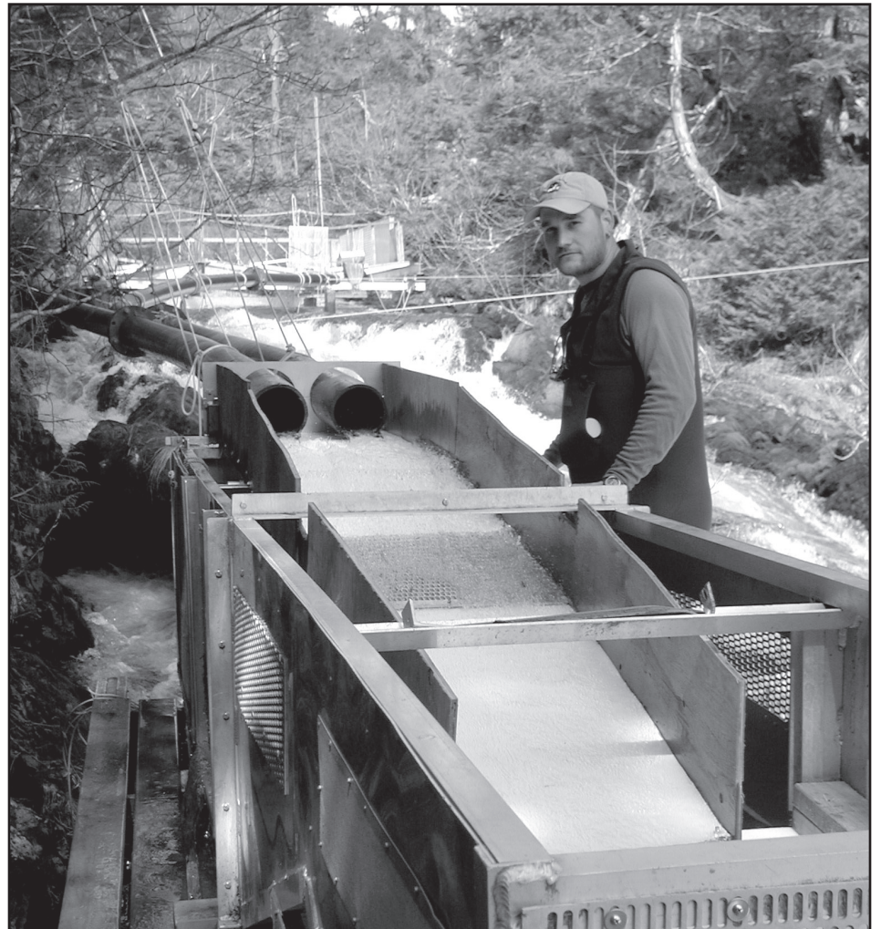
Josh Homer, Deer Lake project biologist, adjusts de-watering device this spring. Weir and pipeline in background.
